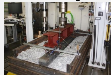
Fatigue test in ballast trough
