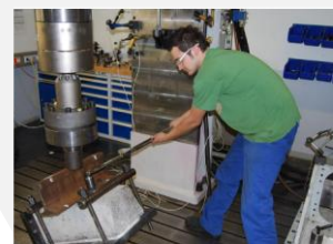
Fatigue test in ballast trough
