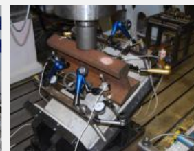
Fatigue test in ballast trough
